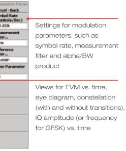
Automated measurements for EVM, Magnitude Error, Phase Error, plus symbol number where each measurement peaks
